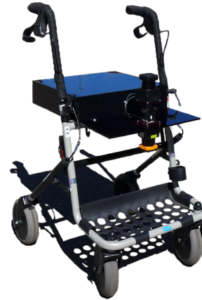
Fig. 1. The smart walker is an off-the-shelf walker retrofitted with an extension unit that contains computing capabilities and two laser scanners for perception. Additionally, two vibration motors are integrated into the handles for tactile feedback generation.
