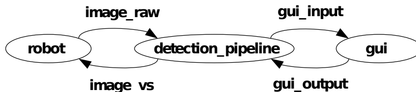
Figure 6.1.: Network topology of the weed detection pipeline. The ellipses are ROS nodes which can be run on different machines. They communicate by ROS topics.
