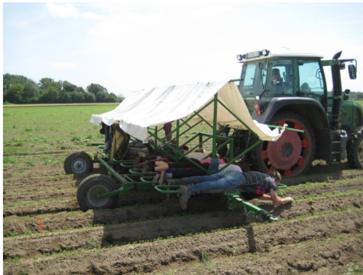
Figure 1.1.: State-of-the-art weed regulation technique for organic carrot fields in Germany
