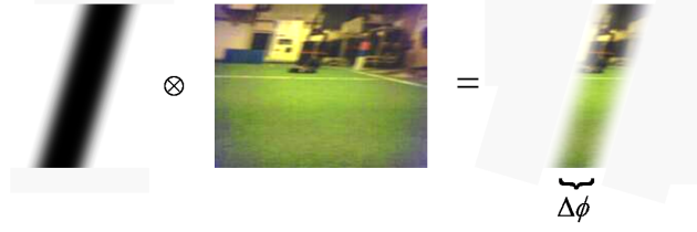
Figure 3.2: The image is scanned in vertical direction for color class transitions at an angular resolution of \Delta\phi by the convolution with a Gaussian stripe.
