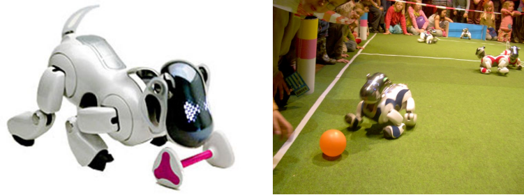
Figure A.1: Sony's Aibo entertainment robot, series ERS7. Left: The Aibo's default software (Aibo Mind) lets the Aibo play with its pink bone. Right: Soccer playing Aibos of the Dutch Aibo Team (picture taken at the Cinekids Festival 2005, Amsterdam).
