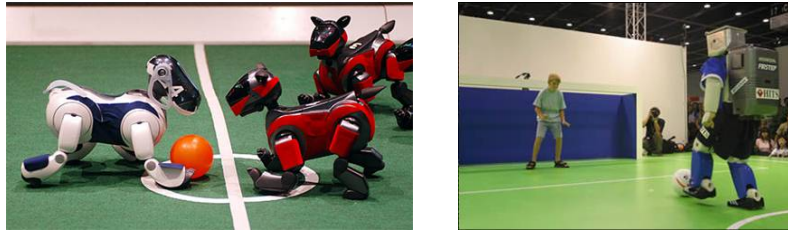
Figure 1.1: Pictures taken at the RoboCup competitions. Left: 4-Legged league, Aibo ERS210 and ERS7, a few seconds after kickoff. Right: Honda's Asimo, demonstrating its abilities by shooting penalties against a human goalkeeper.
