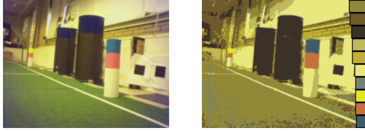
Figure 4.1: Automatic color clustering. Left: Original image. Right: Resulting color class image. The color classes found by the EM-algorithm are listed at the right border.
