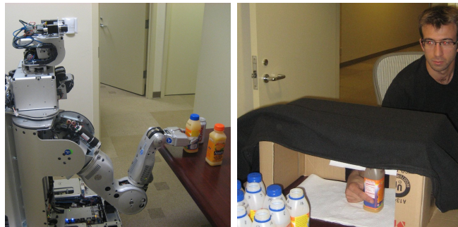
Fig. 1. Left: A mobile manipulation robot grasping a bottle estimates the internal state of the grasped object from its tactile appearance. Right: Comparative study on tactile performance with human test subjects.
