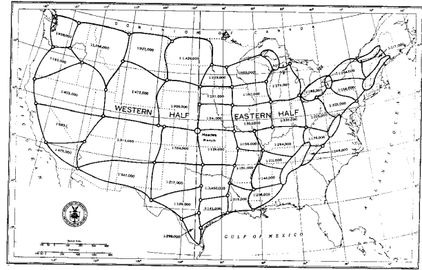
Fig. 3. Bowie method as used for NAD 27 triangle net (left) and the resulting approximation (right). Each small circle represent a junction and the junctions are connected by sections. Given the values of the junctions, the segments are independent of the rest. Courtesy of [35].
