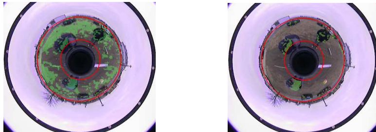
Fig. 3. Omnidirectional camera ROI is defined by the two red circles. Results of color clustering are shown in the left figure, final color blobs in the right figure
