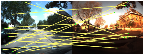
Figure 2: Feature-based matching of the same place across seasons. In this example, SURF features do not match reliably due to a substantial visual change.
