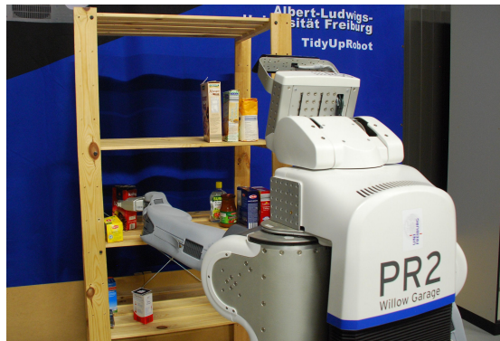
Fig. 1. A robot arranging objects on shelves by predicting user preferences. First, it predicts pairwise preferences between objects, and then it assigns objects to different shelves by maximally satisfying user preferences.
