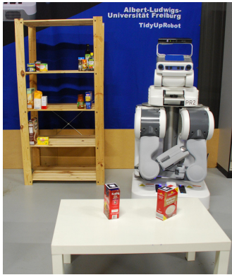
Fig. 9. The robot has to assign the two objects that are on the table to shelves according to predicted user preferences. In this example, the robot places coffee on the same shelf as tea , and rice next to pasta .
