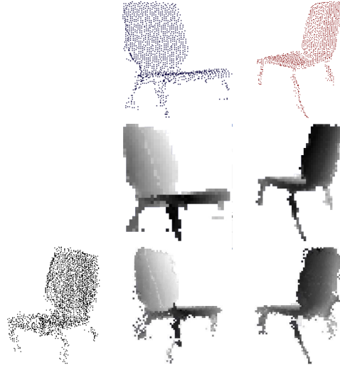
Fig. 5. Two range images generated for evaluating the score of the match. The first row shows two of the original models from two viewpoints. The second row shows the range images extracted from the models at the original viewpoints. The last row shows the model constructed by merging the two original ones and two range images extracted from the combined model at the original viewpoints. These range images will then be compared with the original ones.
