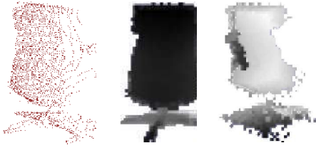
Fig. 2. Example of range images generated from a point cloud. The original point cloud (left) and range images obtained from different viewpoints (center and right). The darker a pixel of the range image is, the closer to the viewpoint.
