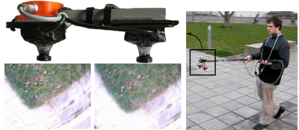
Fig. 1. Top Left: the sensors used for testing our approach. We assembled two cheap USB web-cams as a stereo pair and combined it with a XSens MTi inertial measurement unit. Bottom Left: a typical stereo image used for constructing the map. Note the significant motion blur affecting the image. Right: the procedure for acquiring the data. We mounted the sensors with the cameras looking downwards on a stick and we then walked around the campus.
