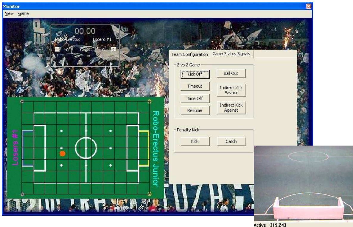
Fig. 2 Human-Humanoid Robot Interaction (HHRI) System of Robo-Erectus Junior Humanoid Robot
