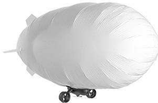
Figure 2.2: Complete blimp selected. The balloon has a size of 52" and at the bottom is the tri-turbofan gondola
