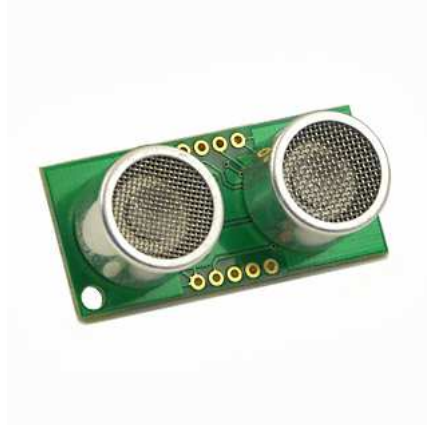
Figure 6.1: We see an ultrasonic sensor SRF05. We used it to get the measurement of the altitude. This sensor weight 10 grams
