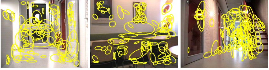
Fig. 5.21. Local patches at the interest points detected in three typical images acquired in an indoor environment. The size of the patches illustrate the scale at which the points were detected.
