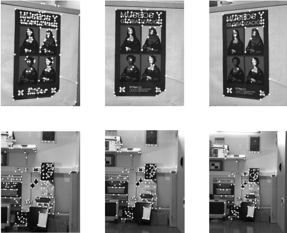
Fig. 4 The top images are examples of a planar object under different changes in viewpoint. The bottom images depict a 3D scene under different scales. These are the first, the central and the last image of a sequence of 21 images (viewpoint transformation) and of 12 (scale transformation). The tracked points are indicated by white marks.
