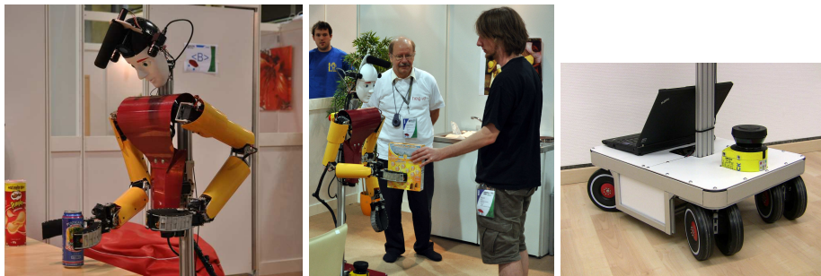
Fig. 2. Our domestic service robot Dynamaid with anthropomorphic arms and omnidirectional base.
