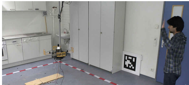
Fig. 1. Our approach enables a quadcopter to follow a person and to understand simple gesture commands such as “follow me”, “take picture”, and “land”.
