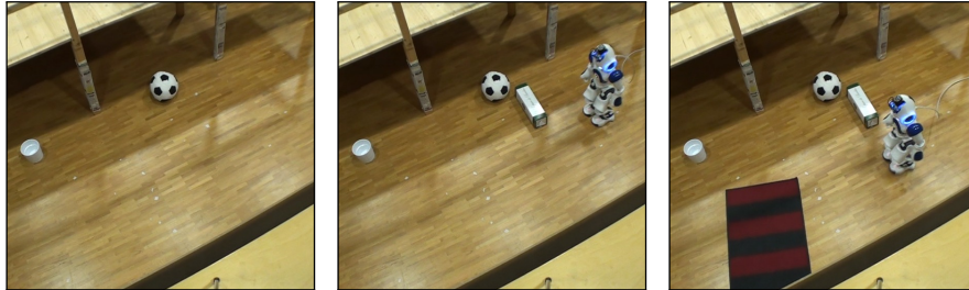
Fig. 15. Left: Scene during training (robot outside the camera's field of view). Middle: New but similar-looking objects do not trigger retraining. Right: The newly appeared carpet is correctly interpreted as a substantial change and retraining is triggered.
