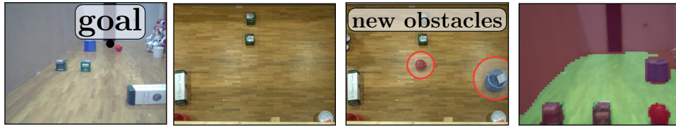
Fig. 7. Left: scene from the robot's view, 2 nd left: top view, 3 rd left: scene changed while navigating, right: labeled image from the robot's camera.
