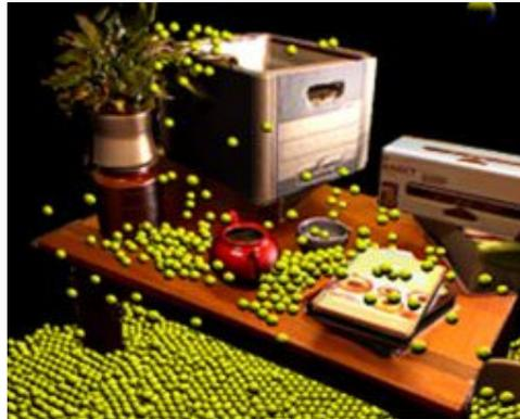
**Figure 1.2.:** KinectFusion: A related approach for precise 3D reconstruction in real-time. It also allows an augmented particle simulation [23].
