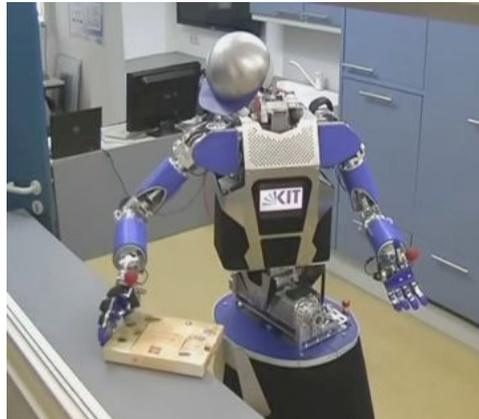
**Figure 1.3.:** Pushing an object to enable grasping: Since the manipulator is not able to grasp it directly, the robot pushes it to the edge of the table for grasping. The physical parameters are initially unknown and learned by a series of manipulations [34].
