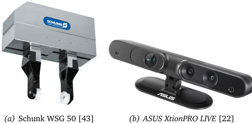
**Figure 5.2.:** The gripper allows stable pushing of objects. The RGB-D sensor from ASUS provides point clouds, color and depth images.
