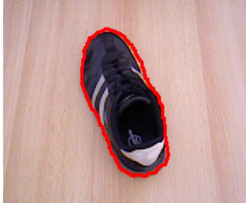
**Figure 3.7.:** The projection of the current object model into the color image yields the segmentation of the image.
