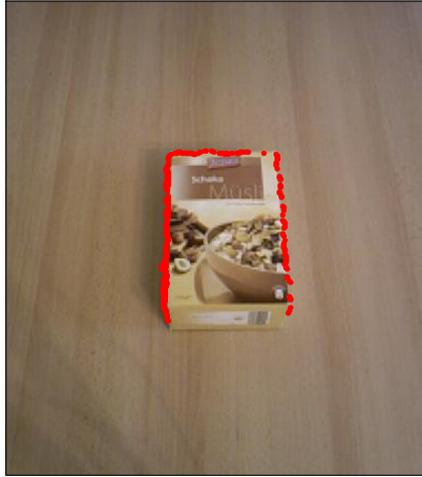
**Figure 3.6.:** Noisy points of a point cloud: The red dots correspond to points, which have an above-average variance in depth across several sensor readings. We ignore these points in further computation steps to avoid false positives in the change sets.
