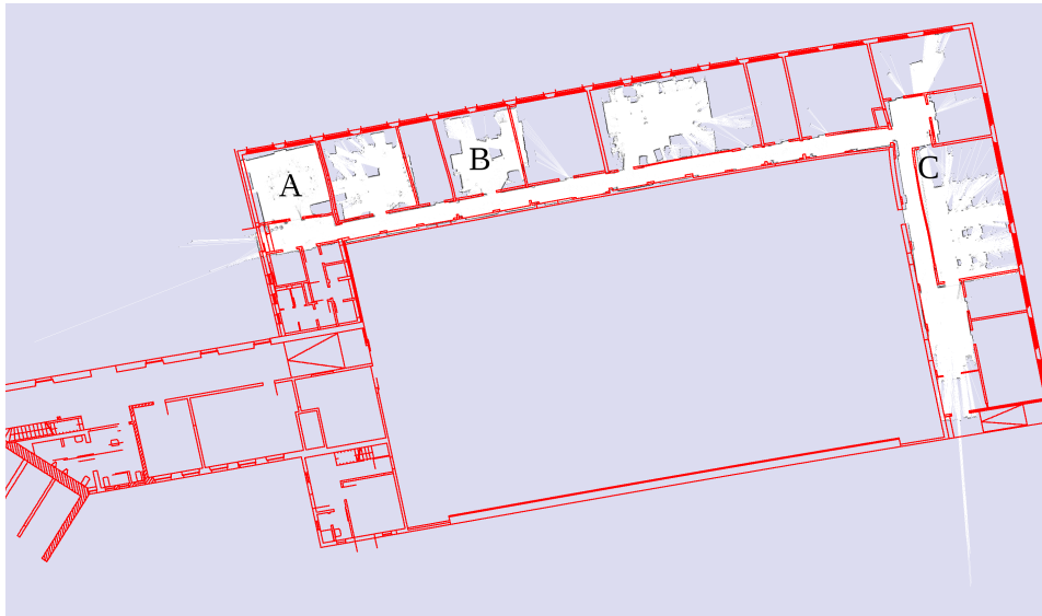
Figure 6.2.: The floorplan is mapped onto the gridmap through a combination of transformations.
