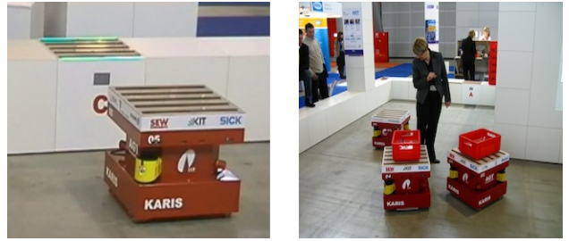
Fig. 2. The target system: Robots equipped with conveyor and RFID reader for autonomously handling transportation tasks: (a) approaching a station for loading. (b) safe navigation among humans.
