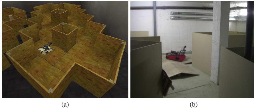
Fig. 10. (a) shows the simulated Matilda in USARSim, based on the Unreal2004 game engine. (b) shows a part of our real-world test arena.
