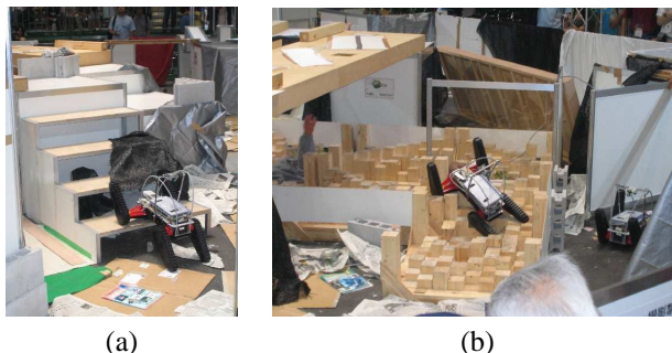
Fig. 1. The Lurker robot during the RoboCup Rescue competition in Osaka. (a) climbing stairs and (b) searching for victims in a large random stepfield.
