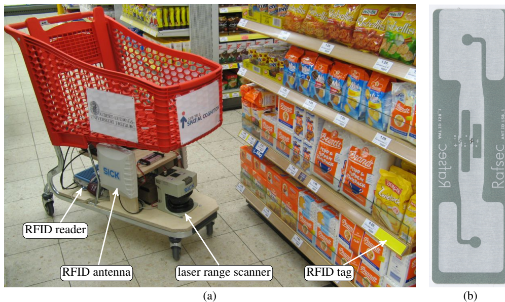
Figure 3.5: (a) We equipped a shopping cart with an RFID reader and a laser range scanner and deployed about 350 passive UHF tags in a supermarket. (b) DogBone RFID tag by UPM Raflatac.
