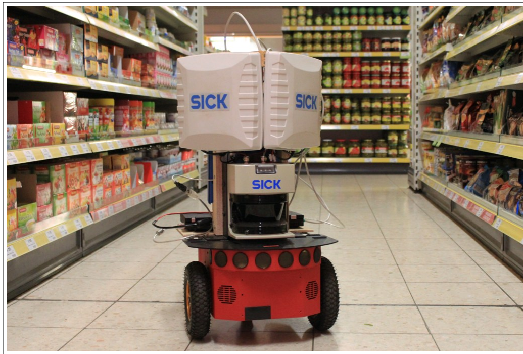
Figure 1.1: A first contribution of this thesis is a technique for object localization. As future household objects and retail products may already be equipped with RFID tags, we propose a novel approach to RFID-based localization and mapping.
