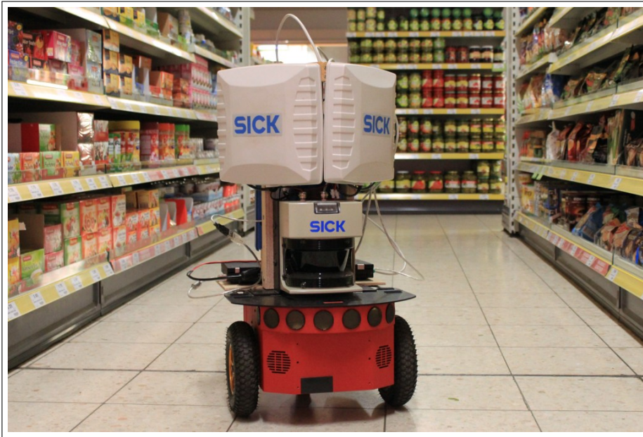
Figure 4.12: We equipped a Pioneer 3DX with a SICK laser range scanner and a SICK RFID reader with two antennas. The robot autonomously searched for a product in a supermarket using our proposed search strategy.
