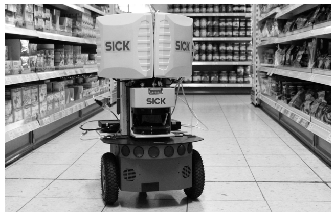
Figure 8: We equipped a Pioneer 3DX with a SICK laser range scanner and a SICK RFID reader with two antennas. The robot autonomously searched for a product in a supermarket using our proposed search strategy.
