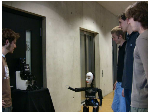
Fig. 1. Robotinho guides visitors to exhibits and presents them. It uses multiple modalities to interact with people in a natural way.
