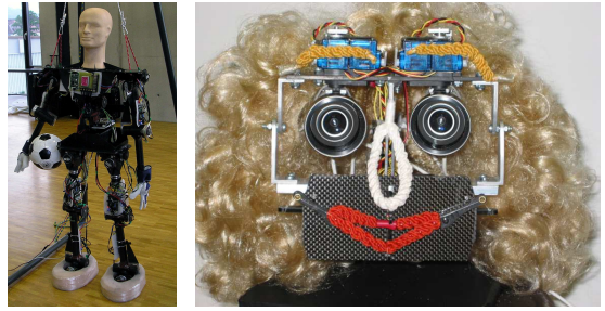
Fig. 2. The left image shows the body of our robot Alpha. The image on the right depicts the head of Alpha in a happy mood.
