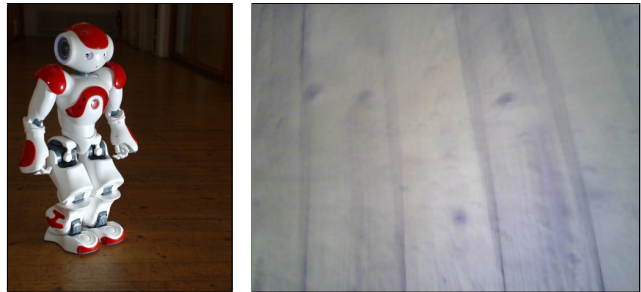
Fig. 1. The Nao robot [1] walking in our corridor environment (left). The robot observes floor patches from which it extracts features for localization. While walking, significant motion blur is introduced in the captured image (right), resulting in non-detection of features.
