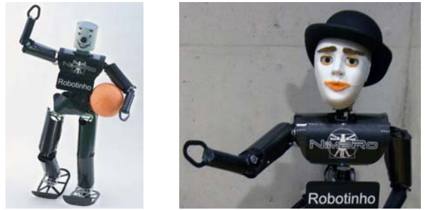
Fig. 1. Our robot Robotinho was initially used as soccer player in the RoboCup Humanoid League. Recently, the robot was equipped with a 2DOF neck and a 15DOF communication head.
