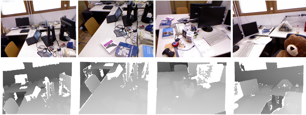
Figure 3.2: Color and depth images as obtained by a Microsoft Kinect. Comparable data is obtained from the Asus Xtion Pro Live. The gray levels represent the distance of the depth image. White corresponds to the absence of a measurement.
