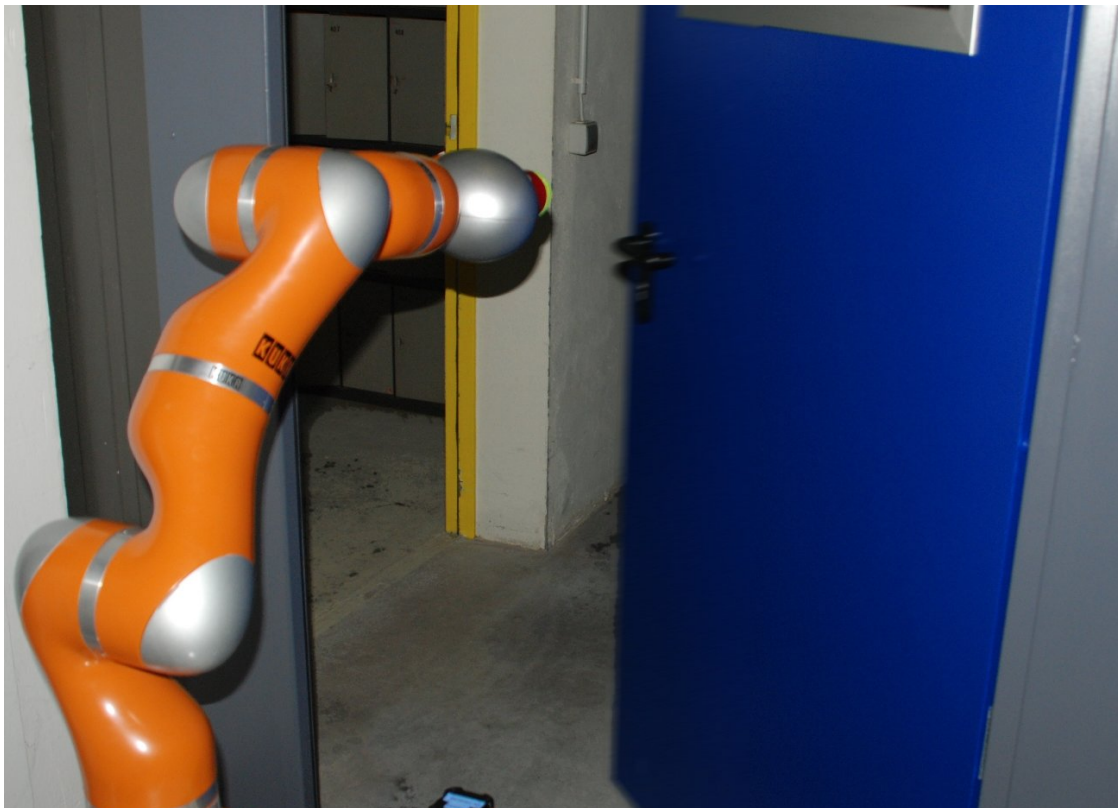
Figure 5.7: The DLR Light Weight Robot with custom end effector used in our experiments, opening the metal door.
