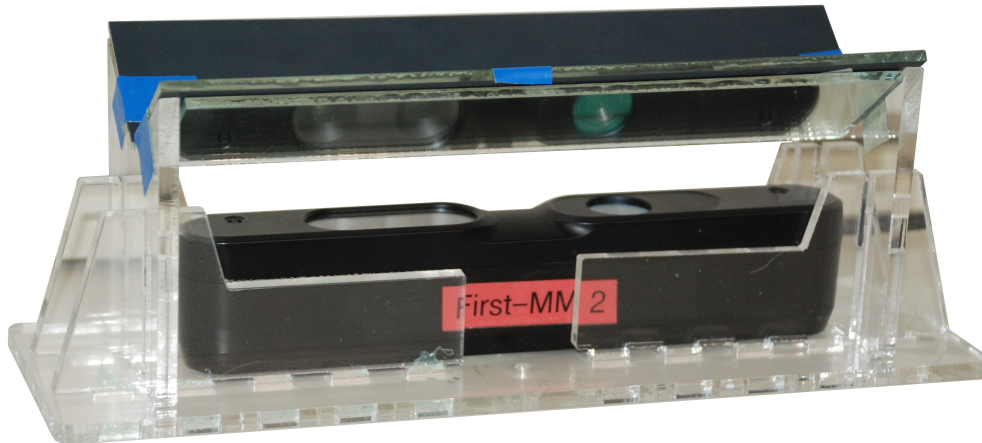
Figure 4.4: The assembled catadioptric sensor using an Asus Xtion PRO Live, two mirrors and a mount made of transparent acrylic sheet. Figure 4.5 depicts the CAD model of the mirror mount.
