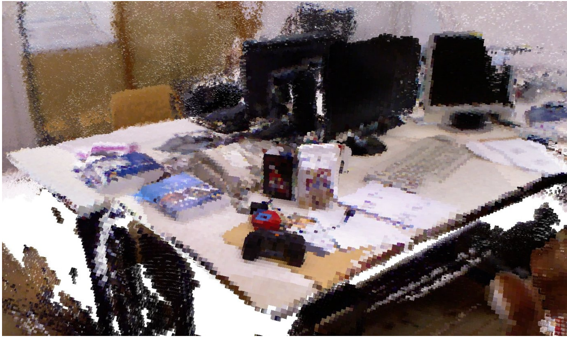
Figure 3.5: Occupancy voxel representation of the sequence “fr1 desk” with 1\text{ cm}^3 voxel size. Occupied voxels are colored for easier viewing.
