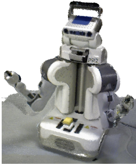
Figure 3.6: Occupancy voxel map of the PR2 robot. Voxel resolution is 5 mm. Occupied voxels are colored for easier viewing.
