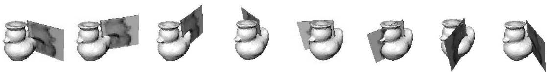
Figure 3.6: Eight steps in the generation of a spin image on the model of a rubber duck. Image taken from (Johnson, 1997)
