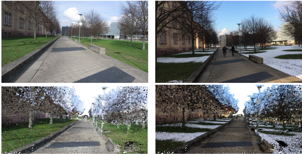
Fig. 3. Top: Example camera images from the Freiburg campus dataset. Left: A day without snow captured with a Canon S100 compact camera. Right: A snowy day captured with the camera of an Apple iPhone 5S. Bottom: Post-colored point cloud from a similar point of view. As can be seen, very fine structures like thin tree branches tend to be colored incorrectly (with sky texture). This is related to the localization accuracy but also caused by inaccuracies of the 3D map.
