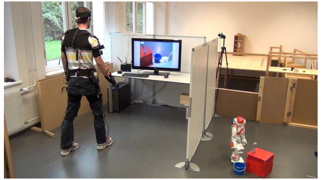
Fig. 10. Tele-operation with visual feedback. Left : Human operator and live view of the robot’s camera displayed on a monitor. Right : Tele-operated Nao humanoid.
