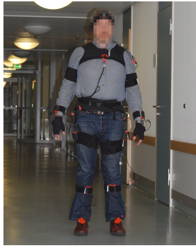
Fig. 2. XSens MVN motion capture suit used to record motions of healthy and PD subjects performing clinical experiments.
