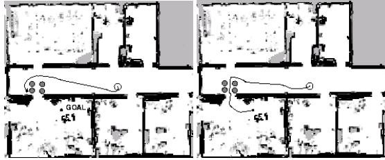
Figure 5: Albert tries to enter a doorway blocked by several obstacles using the DWA (left) and our technique (right).
