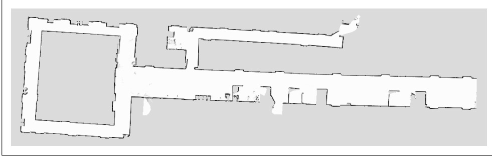
Figure 1. Two-dimensional map of Sieg Hall at University of Washington, Seattle, constructed out of 8013 2d range scans.
