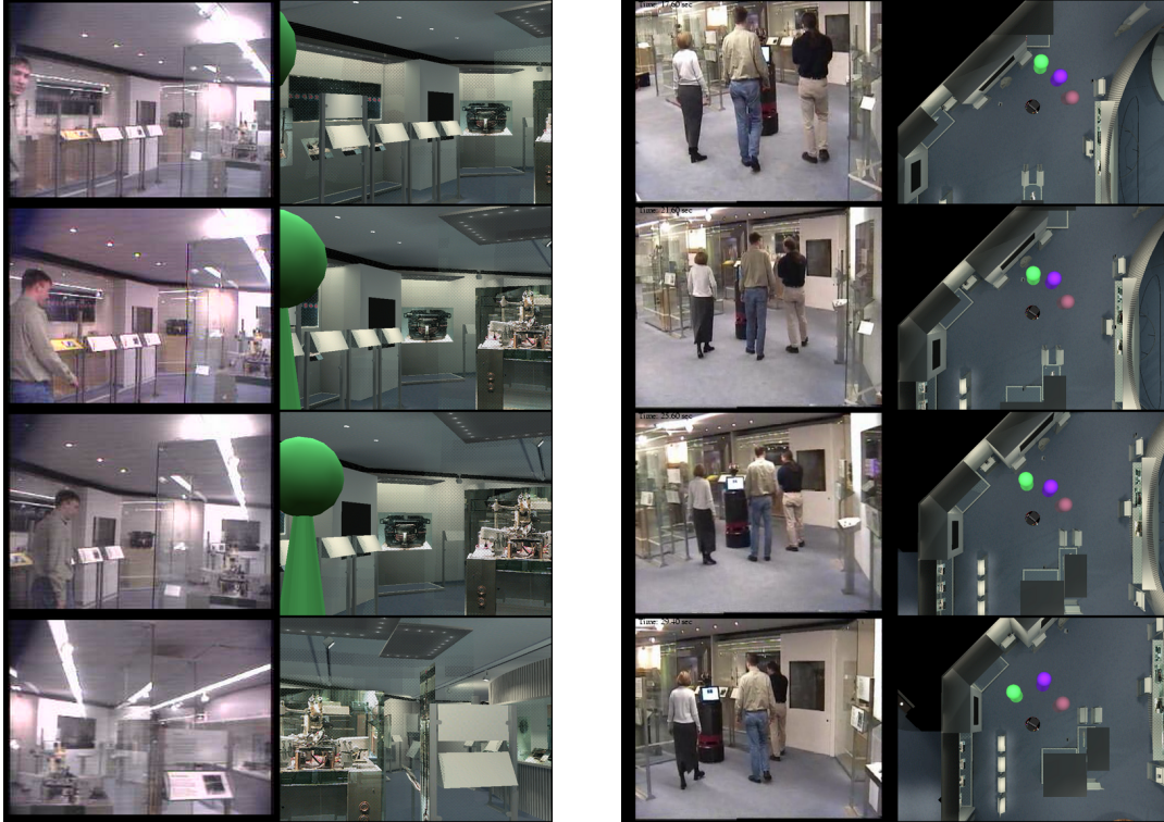
Figure 5. The enhanced 3D visualization allows arbitrary view-points. The left sequence shows the real and the virtual view through the robot's cameras. The right images show the robot guiding three people through the museum and a bird's eye view of the scene.
