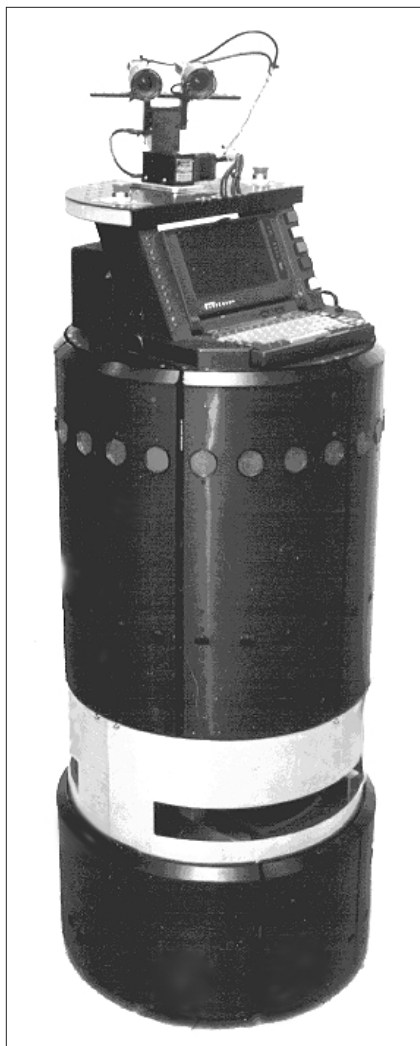
Figure 1. Rhino, an RWI B21 mobile robot, has a unique control system enabling successful operation in increasingly complex environments.
