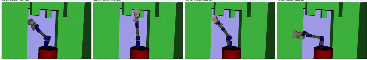
Fig. 5. Path of the manipulator generated by the path planner in a simulated environment.
