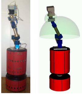
Fig. 1. Robotic platform (left) and simulated robot including the configuration space of the manipulator (right).
