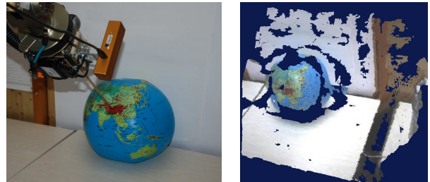
Fig. 1. Deformation of an object in reality (left) and the 3D perception of the robot (right).
