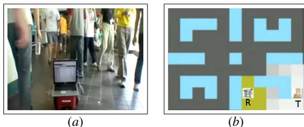
Fig. 1. Different scenarios: (a) Crowded canteen environment : Highly dynamic and unknown environment, suitable for local planning (b) Home care application : Uncertainty in target’s position handled by POMDP tracker can generate sophisticated behaviors.
