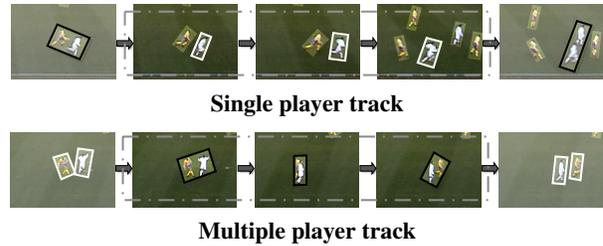
Figure 1. **Single and multiple target tracks** from a football game. The top row shows a single target track, shown in white. The bottom row is a multiple target track, shown in black. Tracks are sandwiched between interactions with other tracks. During a track the number of targets involved and their identities remain fixed.
