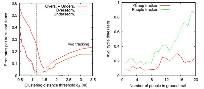
Fig. 5. Left: clustering error of the group tracker compared to a memory-less single linkage clustering (without tracking). The smallest error is achieved for a cluster distance of 1.3 m which is very close to the border of personal and social space according to the proxemics theory, marked at 1.2 m by the vertical line. Right: average cycle time for the group tracker versus a tracker for individual people plotted against the ground truth number of people.
