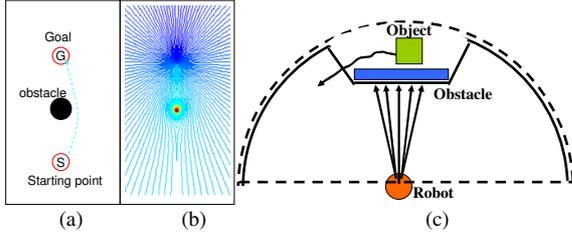
Fig.2. An example of a real environment and its virtual stream field. (a) Obstacle avoidance. (b) Stream field. (c) Real environment.
