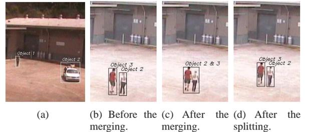
Fig. 4. Multiple object tracking (left). Merging and splitting of two people in a scene (right).
