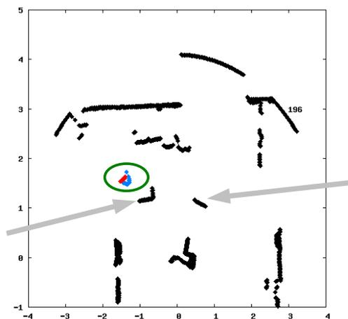
Fig. 6. The image shows an example of a detection for the experiment called *Occlusion* in Table I. The meaning of the colors are the same as in Figure 5. The position of the bins are pointed with light grey arrows. The person is behind one of the bins with his legs occluded. The lasers are located at  $(0, 0)$ .
