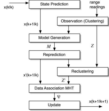
Fig. 2. Flow diagram of the tracking system. See explanations in section V.
