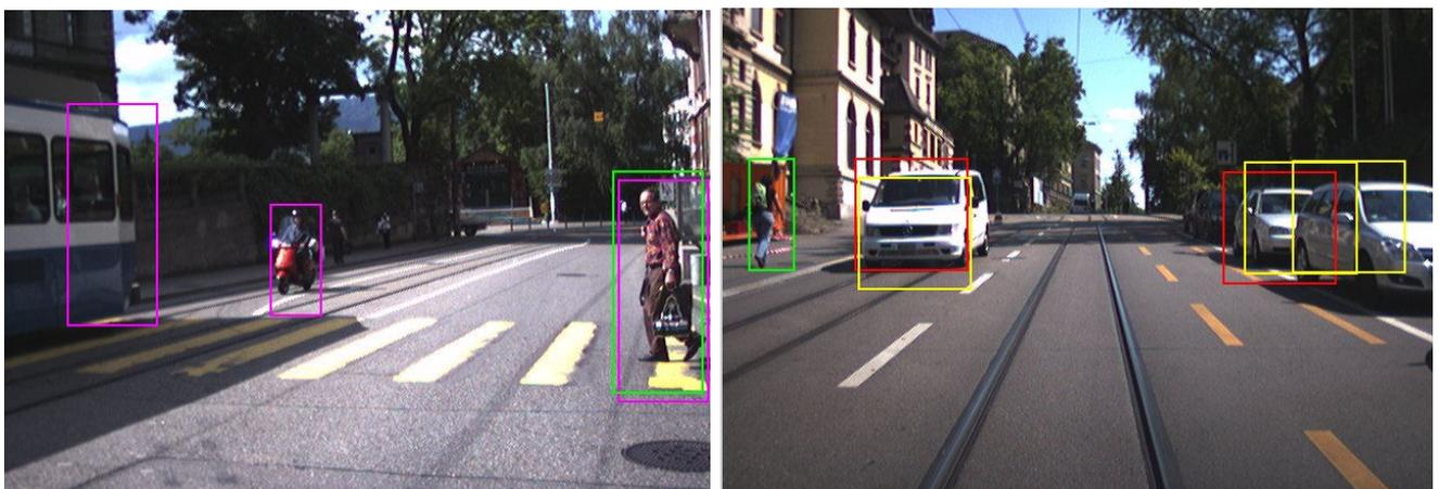
Fig. 4. Detections from multiple sensors. Green: laser based pedestrian detections; Yellow: laser based car detections; Magenta: camera based pedestrian detection; Red: camera based car detection
