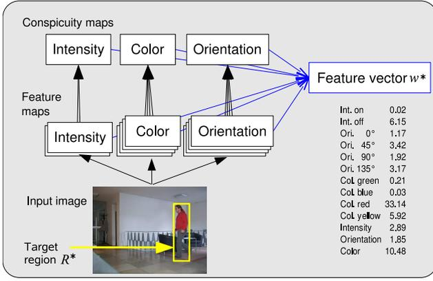
Fig. 1. Initialization: the attention system VOCUS learns the target appearance by computing feature and conspicuity maps for the image and determining a feature vector  $\mathbf{w}^*$  for the manually provided search region  $\mathbf{R}^*$  (yellow rectangle).
