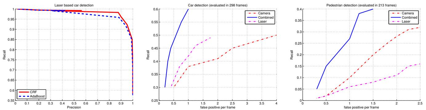
Fig. 3. **Left:** Precision-recall graph for laser range data based car detection. Performance comparison is shown between CRF and a Boost based approach. **Middle:** Recall-false positive per frame for camera-laser information fusion for car detection. A comparison of camera and laser is shown in figure. **Right** Recall-false positive per frame for camera-laser information fusion for pedestrian detection. A comparison of camera and laser is shown in figure.
