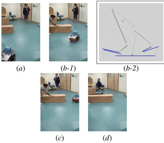
Fig. 5. Vantage tracker : (b-2) shows the robot's local perception of the environment. The target is marked by  $T$ , the blue lines are the occlusion edges, red line is the most critical occlusion and the green segment starting from  $R$  denotes the robot's motion decision. The robot sees the target too close to the occlusion and swings out.
