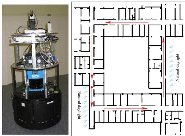
Fig. 2. Left: the RWI B21 robot *Blücher* used for the experiment. The images were taken using the small pantilt mounted webcam on top of the robot. Right: An outline of the environment used for the experiments. The robot tracked the person through the indicated round trip tour (red arrows) and encountered different lighting conditions on its path. The start and end location is marked with a small red circle.
