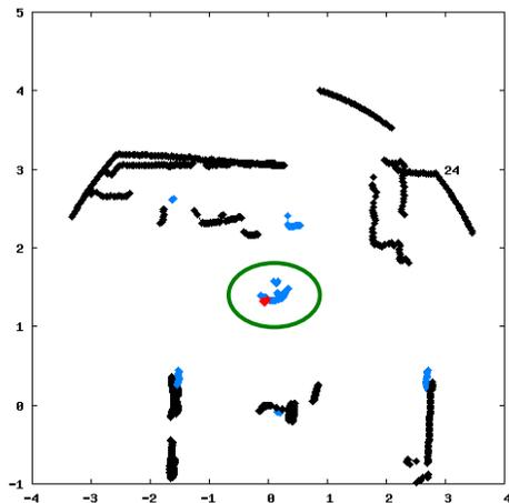
Fig. 5. The image shows an example of a detection for the experiment called *Test* in Table I. Different colors indicate different classifications. Blue segments are classified as body parts, the red segment is the one with best evidence of been a person. Black segments are classified as other objects. The segments corresponding to the person (ground truth) are marked with a green ellipse. The lasers are located at  $(0, 0)$ .
