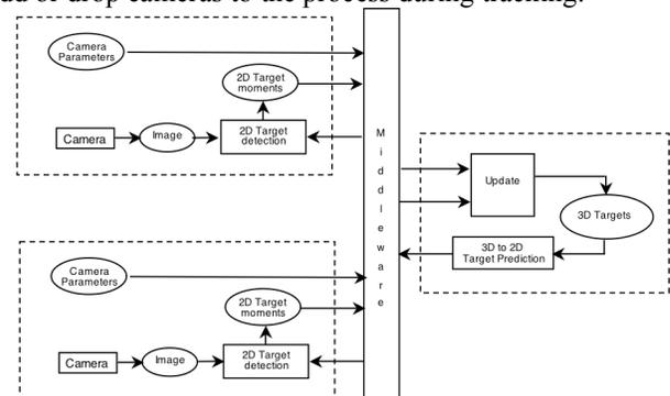
Fig. 3. An example of an assembly of perceptual components. The 3D Bayesian blob tracker provides a ROI and detection method for a number of 2D entity detection components. The result is used to update a list of 3D blobs.
