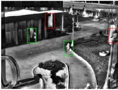
**Figure 5: Sample Test Image fused via Laplacian Pyramid (Green, correct detection; Red, correct rejection)**
