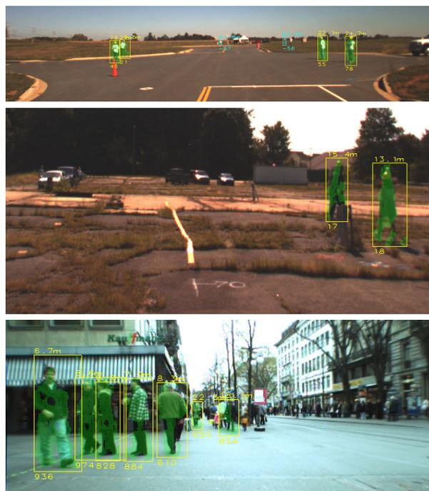
Fig. 1. Examples of test scenarios and the output of our pedestrian detection system (yellow boxes are detections with range and track ID text and a green overlay of the segmented person; the cyan boxes are missed detections).
