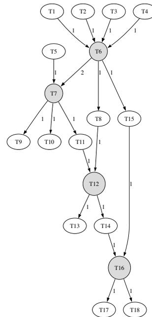
Figure 2. **An example of a simple track graph.** Each node corresponds to a track: white - an individual target, grey - multiple targets. The edges of the graph are directed corresponding to the temporal constraints and indicate when tracks merge or separate.
