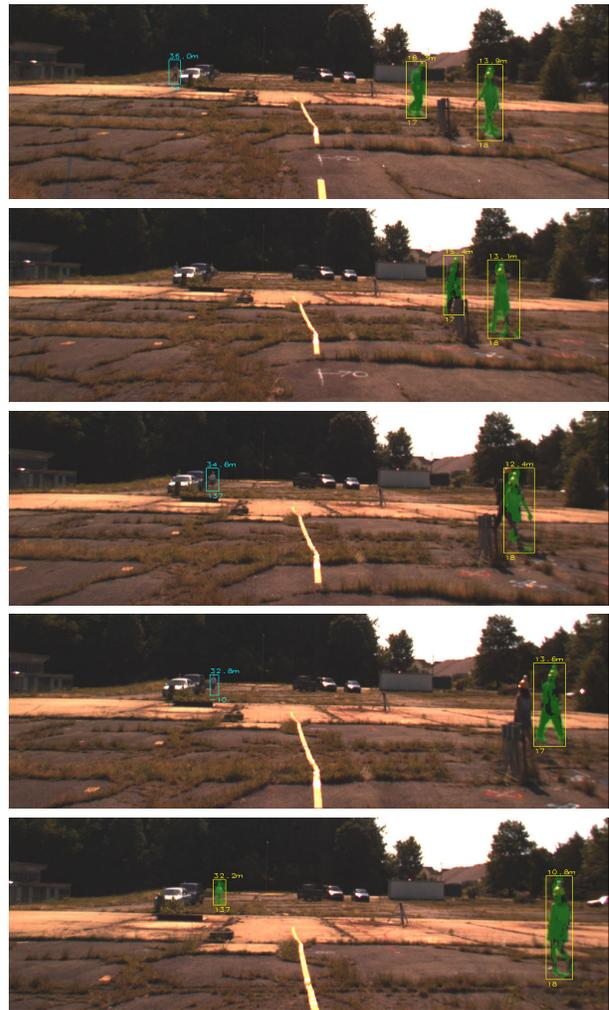
Fig. 5. A sequence of frames showing detections (yellow boxes, with green overlay the segmented person) and misses (cyan boxes) for people under occlusion. The number above the boxes indicates the range, and the number below indicates the track ID.
