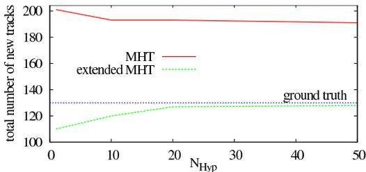
Fig. 5. The total number of tracks as a function of  $N_{Hyp}$ , the number of generated hypotheses. The tracking experiment had 4588 frames with a total of 130 people. The red line shows the MHT approach, the dotted green line the extended approach. The graph shows that replacing the fixed Poisson rates by the ones in the spatial affordance map improves the tracking accuracy significantly.
