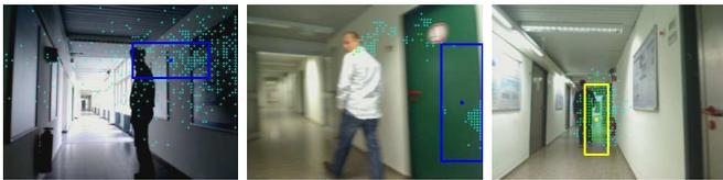
Fig. 5. Failed tracking. The points denote the particles (green points: particles that matched to the target, cyan points: particles that did not match). Rectangles denote the estimated target state (blue: less than 50% of particles match, otherwise yellow).
