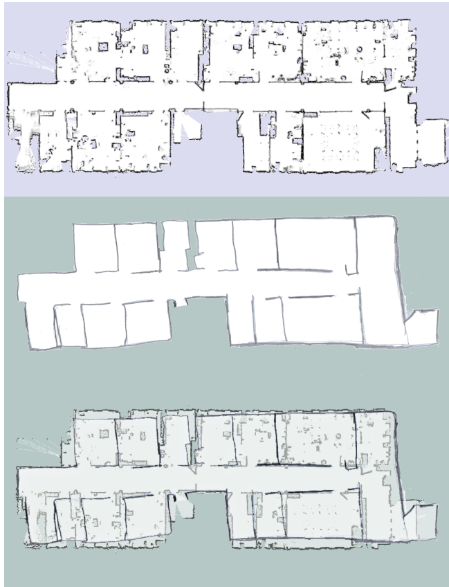
Fig. 1. Occupancy grid of the dataset FR079 (top), built using a SLAM algorithm, a hand-drawn map used to localize the robot (middle) and their overlay (bottom).
