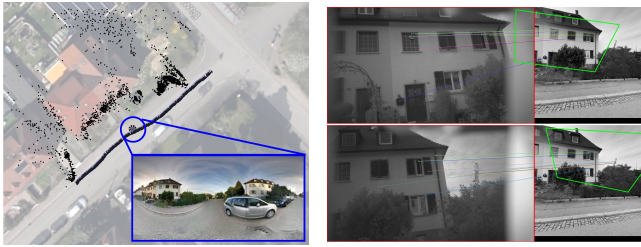
Fig. 10. Optimized 3D points with the estimated panorama position overlaid on Google maps (top). An example of matching between panorama views and Google Tango images. As both cameras are pointing in different directions, the features used internally for visual inertial odometry are different from the features used for localizing Street View panoramas.
