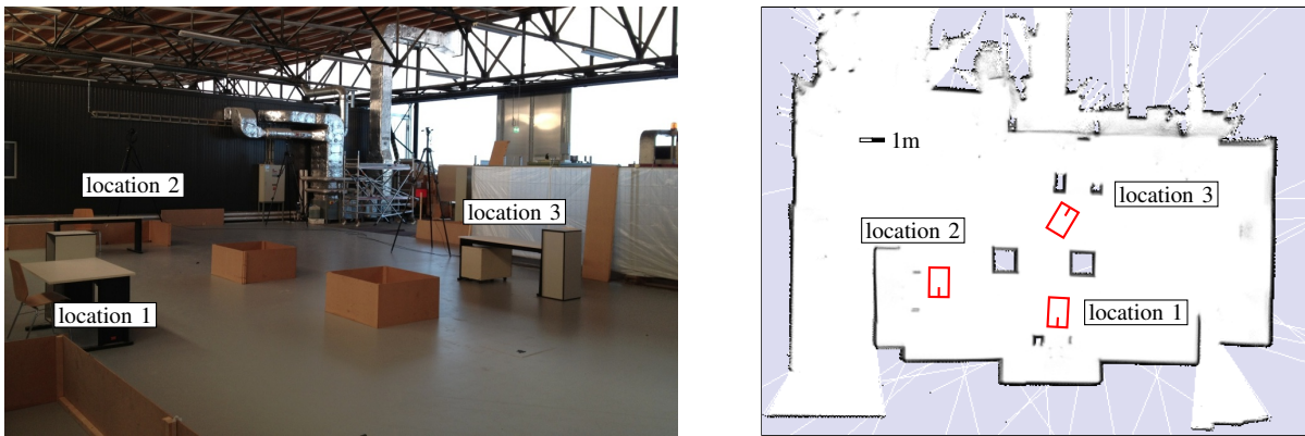
Fig. 3. Left : Evaluation site equipped with a motion capture system. Right : Grid map of the environment with 0.05 m resolution as used for Monte-Carlo localization. Also shown are the three target locations of the platform in front of the work benches.
