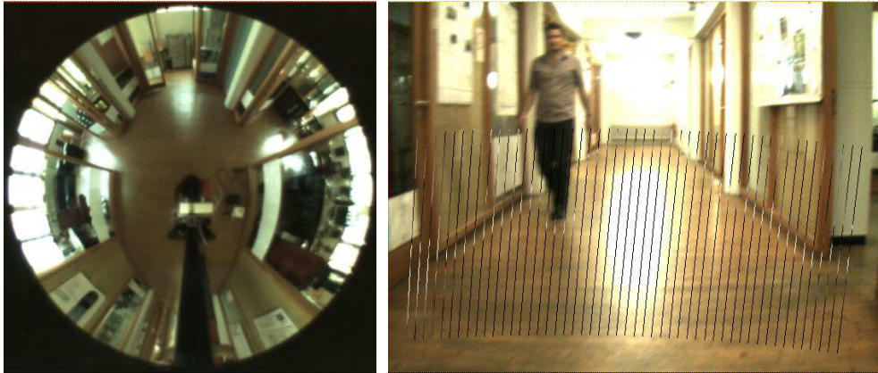
Figure 2: Reflections, glass walls and inhomogeneous surfaces make the relationship between visual appearance and depth hard to model. One of the test environments at the University of Freiburg (left) exhibits many of these factors. Our approach was also tested using a standard perspective camera in this challenging environment (right).
