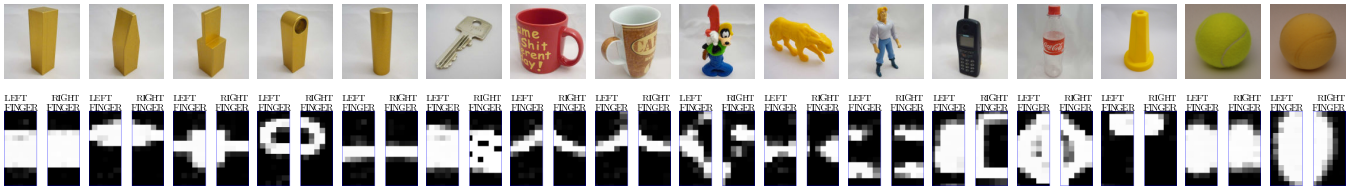
Fig. 4: Various objects used for the experiments. Top row: Visual image of each object Bottom row: Tactile images of left and right finger of each object From left to right: cuboid, triangle, t-object, handle, cylinder, door key, large cup, small cup, goofy, tiger, figure, mobile, bottle, kaleidoscope, tennis ball, and soft ball.
