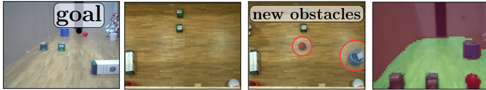
Fig. 7. Left: scene from the robot's view, 2 nd left: top view, 3 rd left: scene changed while navigating, right: labeled image from the robot's camera.
