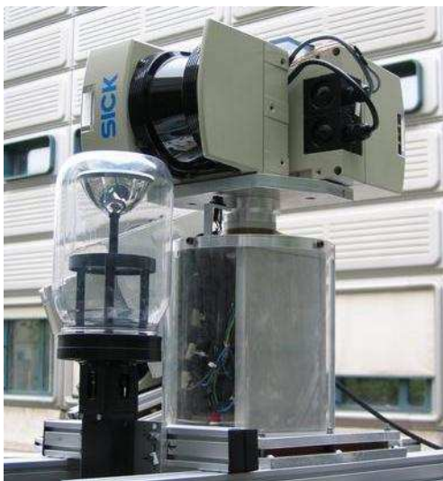
Fig. 5. Rotating scanner and omnidirectional camera
