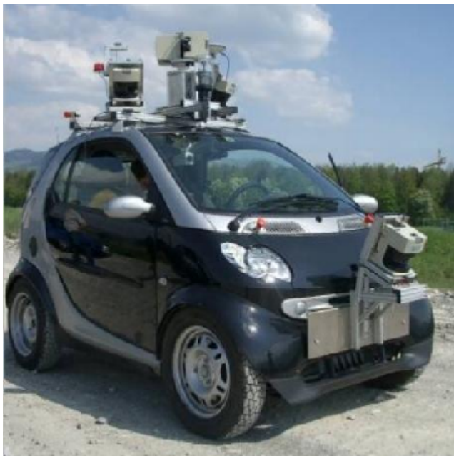
Fig. 1. Our autonomous Smart car platform. There are three fixed laser range finders mounted on the front of the vehicle and on the sides of the roof, and two spinning laser range finders mounted together on the center of the roof. Inside the vehicle, mounted behind the windscreen, is an automotive camera used for lane detection.
