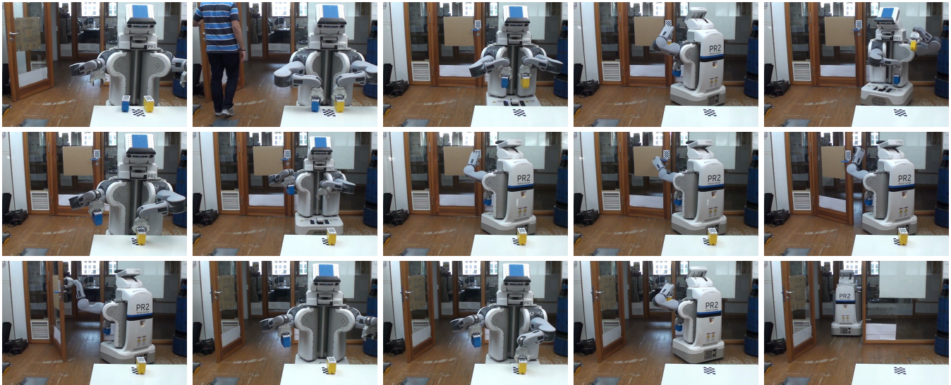
Fig. 5. The robot computes a plan to grasp the two blocks and to bring them outside. Once the robot has grasped the blocks, a person closes the door. After having detected that, the robot computes a new plan and clears its left gripper by first going back to the table and placing the yellow block there. The robot then moves back to open the door and then to the table to regrasp the yellow block. Finally, the robot leaves the room with both blocks and reaches the goal state. See also http://www.informatik.uni-freiburg.de/%7Eabdon/videos/icra13/ for a video of this experiment.
