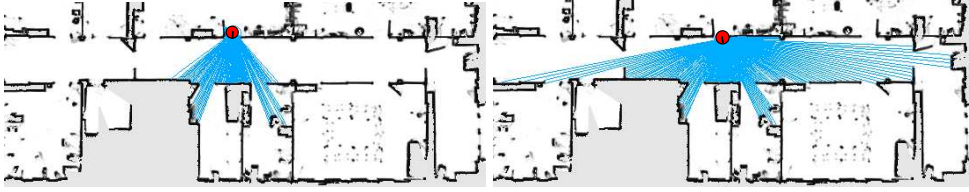
Figure 3.6: In mobile robot localization, small variations in the robot pose can cause large variations of the range measurements. This leads to multi-modal distributions of beam-lengths even in small areas around a potential pose.
