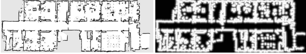
Figure 3.3: Occupancy grid map (left) and likelihood field (right) of the ground floor of building 079 at the University of Freiburg.
