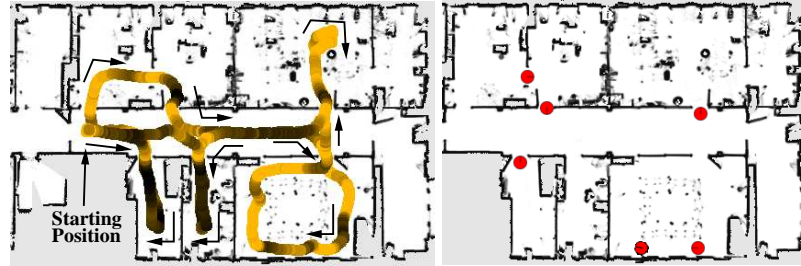
Figure 7.5: The six positions with the highest probability that the global localization in the office environment fails (right). The positions marked in this image directly correspond to the orange positions in the left image. At these positions the likelihoods of the true poses are extremely low due to the multi-modality of the measurements.
