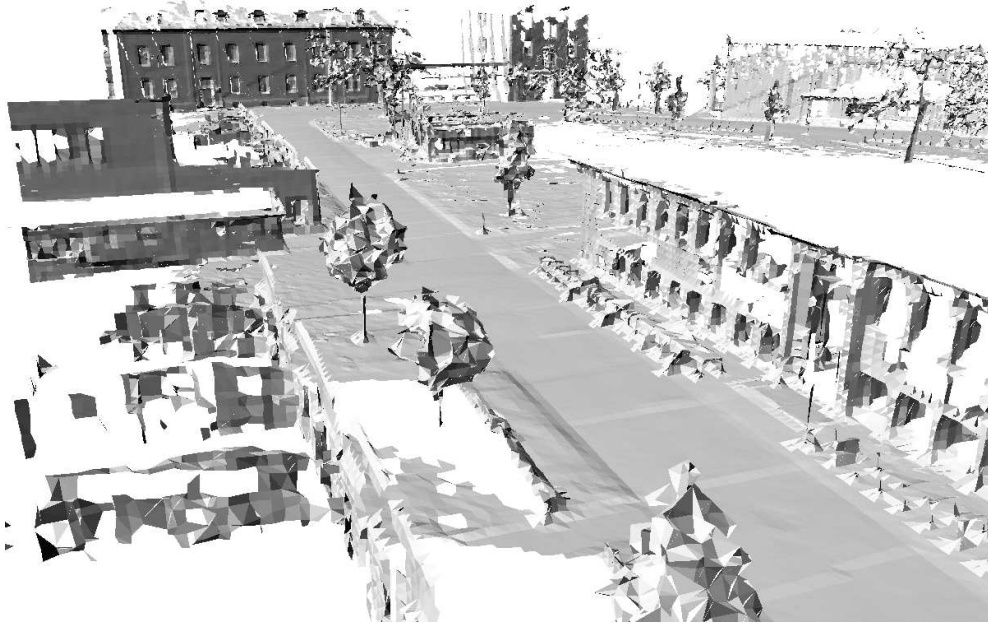
Figure 10.12: Triangulated mesh representation of the outer loop including data points from 77 laser scans.
